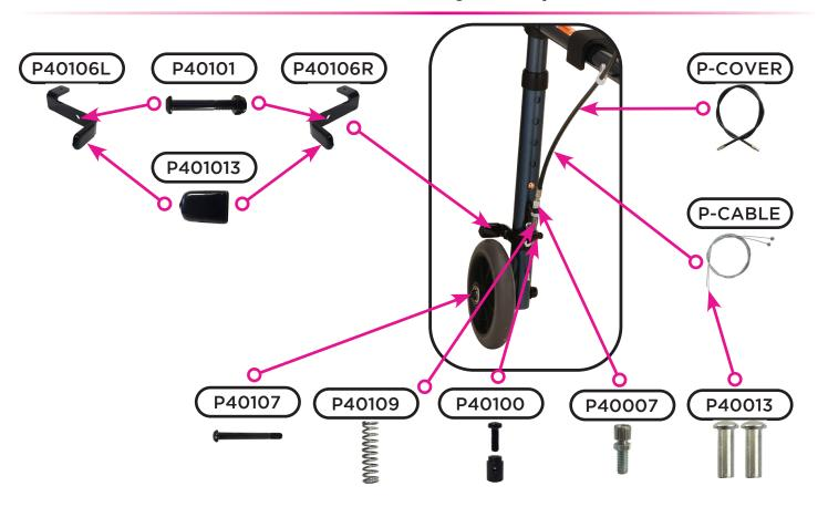
Front Wheel Assembly Components
